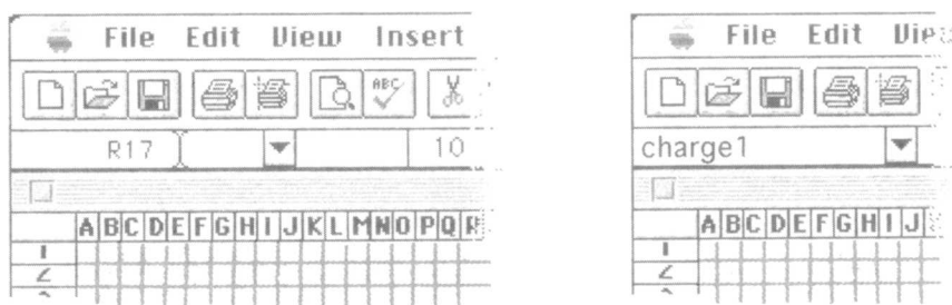
Fig. 2. Click on the naming field and type the name for the cell, in this case charge1. Press the Enter key to complete the cell-naming shortcut.
