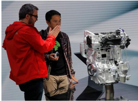
Figure 2 The Infiniti variable compression turbo engine was on display at the Paris Auto Show in September. (Christophe Ena/Associated Press)
