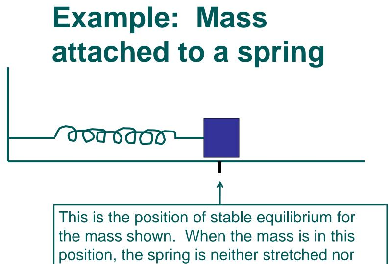
compressed. With the spring in its relaxed state, there is no restoring force.
