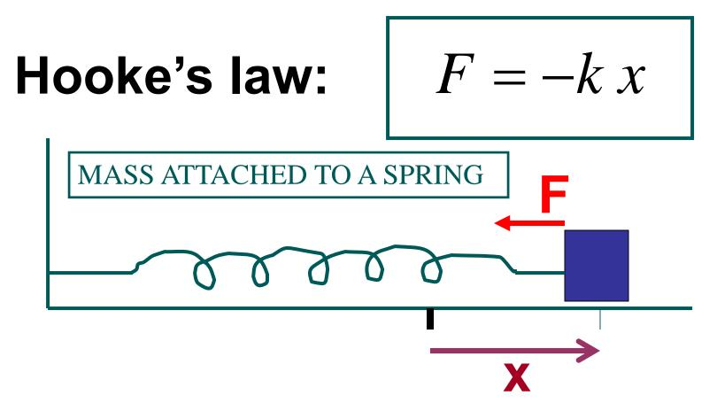
For a spring that obeys Hooke's law, *the magnitude of the restoring force is directly proportional to x*, where *x* denotes the amount by which the mass is displaced from its equilibrium position. (*x* is also the amount by which the spring is stretched or compressed.). See <u>animation</u>.
