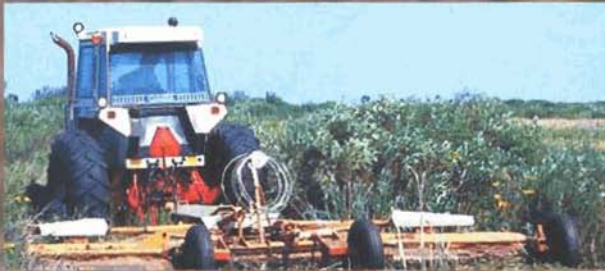
Tractors with big lateral cutters called bat wings mow back shrubs and brush.
